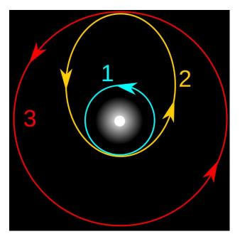
The image shows elliptical Hohmann transfer orbit (2) used by the spaceship. It connects circular orbits of planet B (1) and planet C (3).
